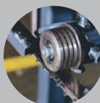
guidance roller arm with electric adjustment
